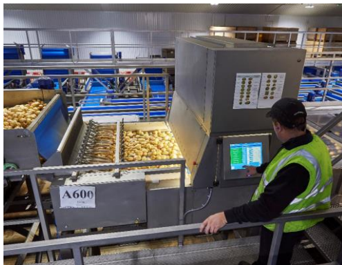
Vision grading the crop to sort the waste from the 1st grade
